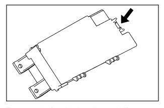
To access the fuse block, pull out and lift up on the cover latch, located at the end of the fuse block, near the battery cable. To reinstall the rear seat cushion, do the following:
